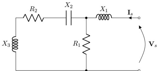
$$\begin{aligned} R_1 &= 48,16 \, \Omega \\ R_2 &= 16 \, \Omega \\ X_1 &= 5,55 \, \Omega \\ X_2 &= -8 \, \Omega \\ X_3 &= 38 \, \Omega \\ Q_{X_3} &= 3800 \, \text{var} \end{aligned}$$
