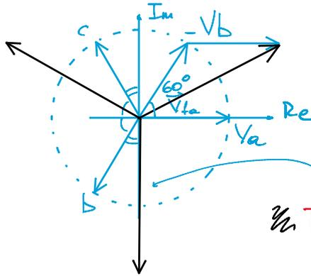
$$\begin{aligned} \rightarrow \text{Da } p(t)_{3F} &= 3V_f I_f \cos(\varphi) \\ &= 3V_f I_L \cos(\varphi) \quad (I_f = I_L) \\ &= \sqrt{3} V_L I_L \cos \varphi \end{aligned}$$
