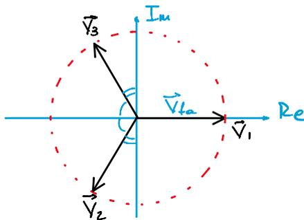
$$\vec{V}_{O'O} = \frac{\vec{V}_1}{Z_1} + \frac{\vec{V}_2}{Z_2} + \frac{\vec{V}_3}{Z_3}$$
